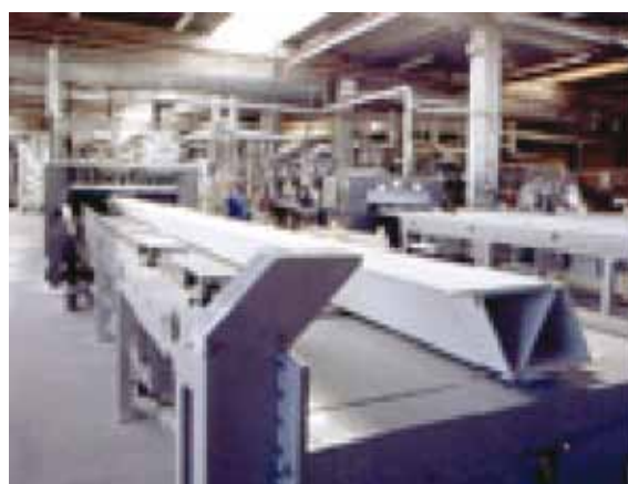
10. Pultrusieprofiel ASSET-systeem. [http://www.fiberline.com/gb/casestories/case3903.asp]
